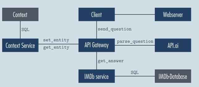
Component diagram of the microservice architecture with aggregate data interface. The atomic variant replaces the IMDb service by separate interfaces for different kinds of requests (get\_movies\_by\_director, get\_movies\_by\_genre,...).
